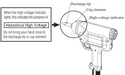
Fig.3-1 Hazardous Points of the Discharge Gun
