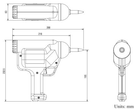
Fig. 8-1 Outline Drawing of Discharge Gun
