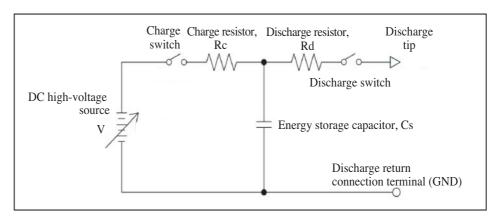
The charge and discharge switches are operated alternately. When the charge switch is on, output from the DC high-voltage source charges Cs via Rc. After charging is complete, turning off the charge switch and then turning on the discharge switch causes the electrical charge stored in the Cs to be discharged to the EUT via Rd.
