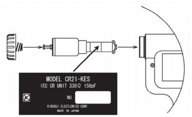
Fig. 2-2 Checking the CR Unit Constant Values
