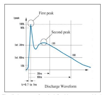
The discharge waveform is defined by current and is determined by the discharge switch and distribution capacity (Cd).\*1 This distribution capacity principally affects the first peak. "Cd + Cs" primarily affects the waveform of the second and subsequent peaks.
