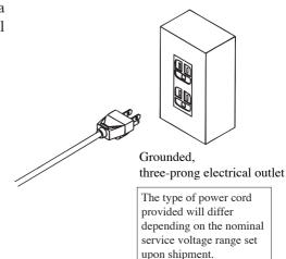
Connect the protective conductor terminal on the rear panel to an electrical ground (safety ground) or otherwise in compliance with the grounding requirements of the Electrical Codes and Regulations applicable in your area.
