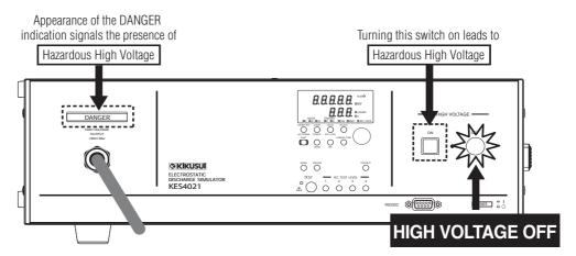
Fig. 3-2 Monitoring the Presence of Hazardous High Voltages
