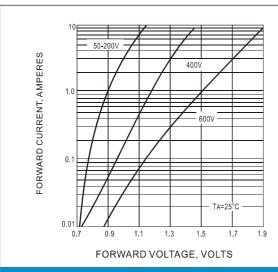
Fig.3 FORWARD CHARACTERISTICS
