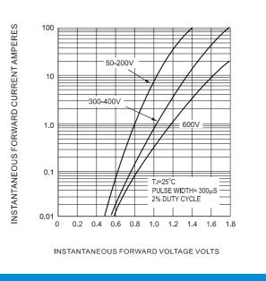
FIG.4 TYPICAL FORWARD CHARACTERISTICS
