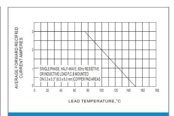
FIG.2 MAXIMUM AVERAGE FORWARD CURRENT RATING
