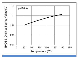
Fig.8 Breakdown Voltage Variation vs. Temperature
