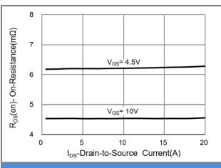
Fig.3 On-Resistance vs. Drain Current
