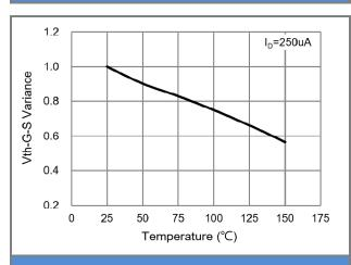
Fig.9 Threshold Voltage Variation with Temperature
