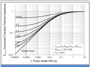
**Fig.12 Normalized Transient Thermal Impedance**
