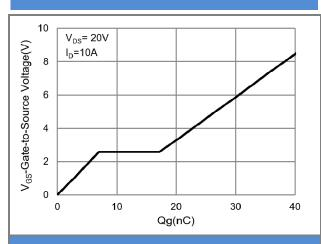
Fig.7 Gate-Charge Characteristics
