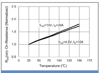
Fig.4 On-Resistance vs. Junction temperature
