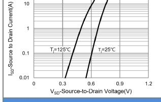
Fig.6 Source-Drain Diode Forward Voltage
