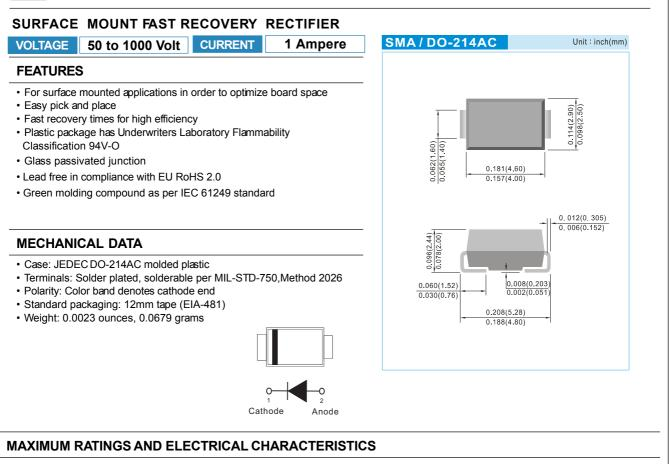
Ratings at 25°C ambient temperature unless otherwise specified. Single phase, half wave, 60 Hz, resistive or inductive load. For capacitive load, derate current by 20%.
