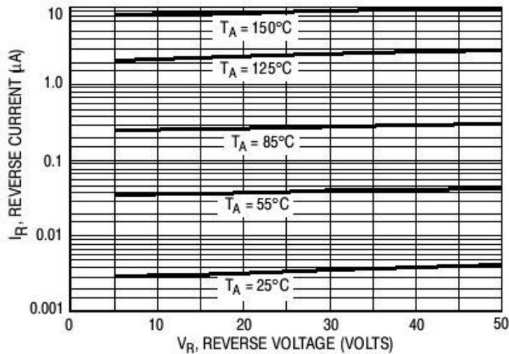
Figure 2. Leakage Current
